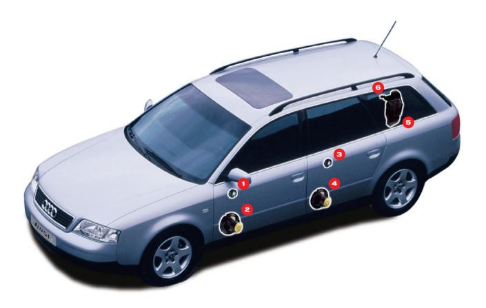
Each part of the Bose sound system has been carefully engineered to work with the others for better performance. Replacing the factory-installed headunit (i. e. radio-CD/navigation system) or any other sound system component will significantly reduce system performance.
